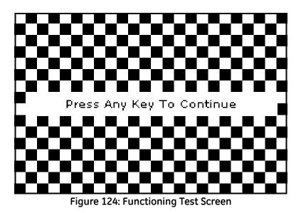
Pressing a key two more times should result in two more checkerboard patterns, followed by a series of dark and light screens. Pressing the key through this sequence should return the PT878 to Operate Mode. If the test does not proceed according to this sequence, please consult the factory.
